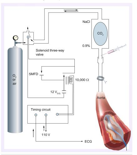
**Figure 4. Counterpulsation device.** The counterpulsation device was pioneered by Moulopoulos *et al.* Timing of inflation and deflation of the balloon was controlled by a Cardiac Programmer manufactured by Cordis Corporation (NJ, USA). A sterile normal saline solution was used to fill the cylinder surrounding the tube to reduce the dead space in the system. The amount of carbon dioxide was regulated with a rudimentary syringe. Reproduced with permission from [18].
