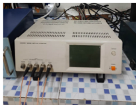
Figure 1. LCR High tester
