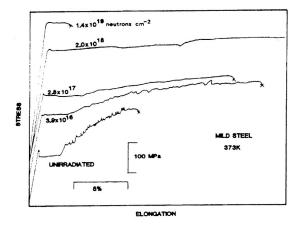
Figure 2: Stress-strain curves of mild steel as a function of neutron fluence
