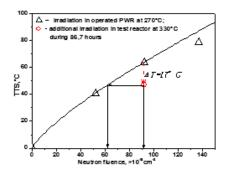
Figure 1: RPV steel TTS dependence on neutron fluence at preliminary irradiation up to ~1020cm<sup>-2</sup> with following extra irradiation at heightened temperature
