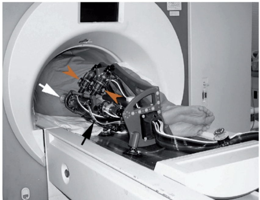
Figure 2. MRBot. Pneumatic stepper motors (arrowheads) and wires (black arrow) orient the end effector for transperineal intervention (white arrow) based on output from the guiding software. Reproduced with permission from [56].
