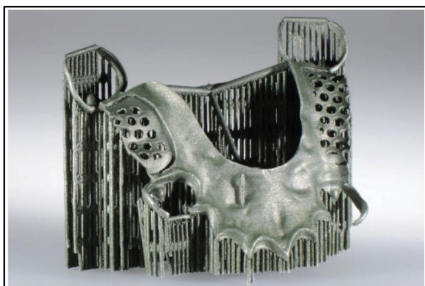
FIGURE 17. Laser sintered removable partial denture with support structure.
