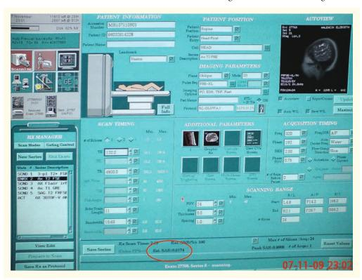
**Figure 3.** The specific absorption rate displayed on the technical console monitor. To avoid potential risks to the fetus specific absorption rate value must not exceed 2 W/kg whole body average.
