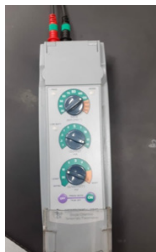
Figure 3: External temporary pacemaker. The sensitivity maintained at 10 mV and output kept at 20 mA with pacing rate of 120 beats per minute.
