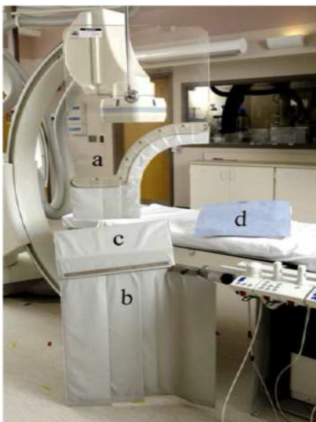
Figure 4. Expanded Shielding System. (a) Large upper body shield with flexible attenuating lamellae, (b) movable lower body shield, (c) vertical extension, (d) disposable radiation absorbing pad to be placed on the patient [65].
