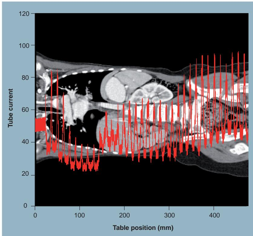
**Figure 1. An example of automatic exposure control in a helical scan.**
