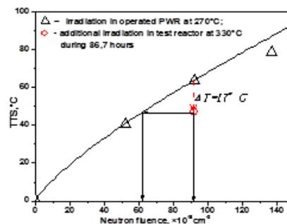
Figure 1: RPV steel TTS dependence on neutron fluence at preliminary irradiation up to ~1020cm<sup>-2</sup> with following extra irradiation at heightened temperature
