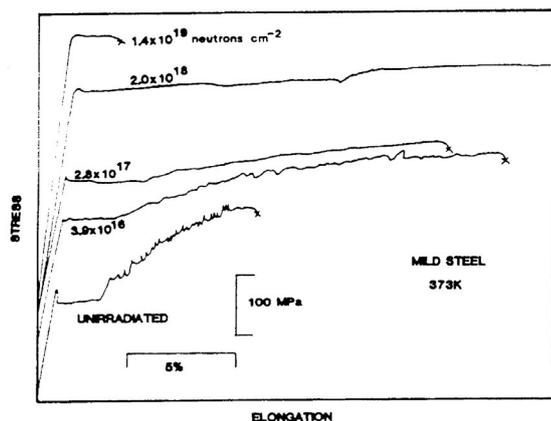
Figure 2: Stress-strain curves of mild steel as a function of neutron fluence
