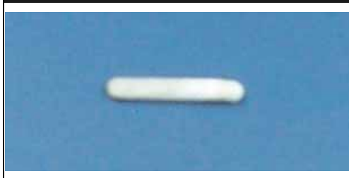
Figure 3. Polylactic acid device after 1 year incubation in dissolution medium.
