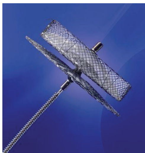
Figure 3. The AMPLATZER® device (AGA Medical Corporation, Golden Valley, MN, USA). The device is made from flexible braided nitinol mesh. Positional forgiveness is achieved through a waist that acts as an articulating, compliant connection between the disc and lobe allowing the disc to self-orient to the cardiac wall.
