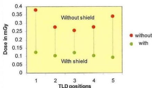
Figure 1a. Dose comparison between doses with and without shielding at individual TLD positions.
